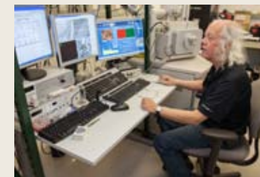
Dr. Richard Piner measuring the composition of a sample with the Oxford EDS system on the FEI Quanta 600 SEM
